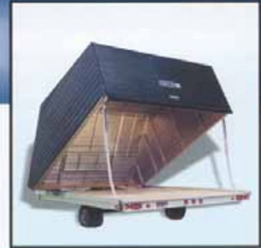
SD 19-10AC-2 in open position showing standard double gas-assisted lift arms
